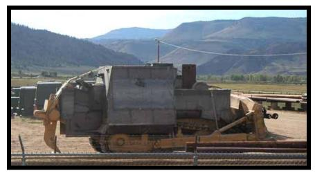
To fit the bulldozer with this shell, Marvin had to use a self-made crane.
